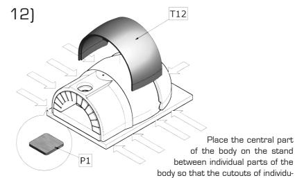
al shaped pieces match and joints are as narrow as possible. If it is necessary to align the parts, place the supplied dilatation pads under the side edges, preferably at places marked by arrows [9 points]. Do not remove the pads. If you use more than 2 pieces of pads on top of each other, bind them together using silicone caulk.
