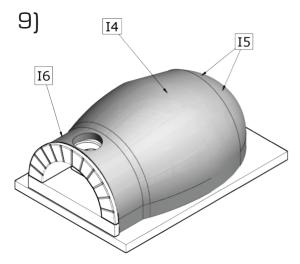
Cover the assembled arch with at least 1 layer of aluminium foil I8. Place the isolation bio-mat on the aluminium foil according to the cutting plan for the bio-mat. Make sure the bio-mat doesn't get distorted during the application.
