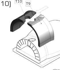
parts, apply adequate amount of silicone caulk into the locks and on the whole surface between the parts. Make sure the caulk don't fill a hole for the thermometer. Maintain a dilatational interstice at least 3 mm between the upper edge of the front arch and the front part of the body. For this purpose place the supplied dilatation pads under the side edges. If you use more than 2 pieces of pads on top of each other,
