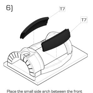
and rear arch. Side arches should be placed with a hole towards the front portal.
